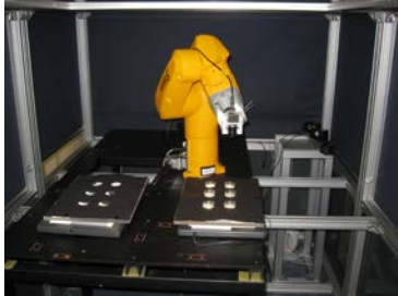
Fig. 29: Robotic video system at EZRC to monitor feeding behaviour of zebrafish
